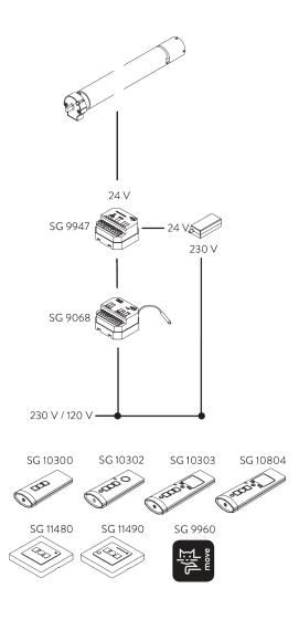
B. WIRING DIAGRAMS Applicable with following systems:
